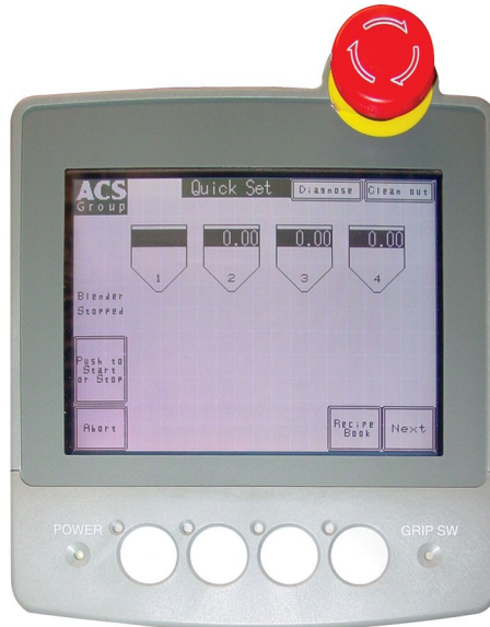
Figure 4: Typical Mitsubishi Controller Touch Screen Display
